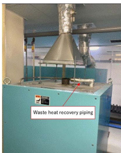
(Equipment Using Waste Heat from Electric Furnaces)
