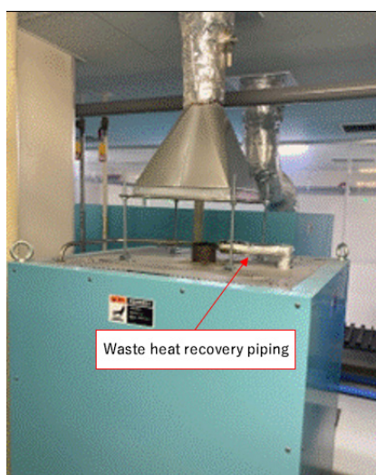
(Equipment Using Waste Heat from Electric Furnaces)
