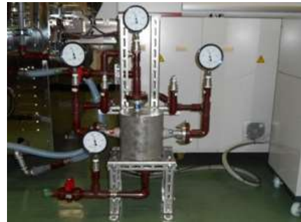
Waste heat recovery heat exchanger (prototype)
